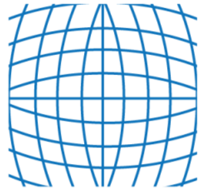
positive radial distortion "barrel"
